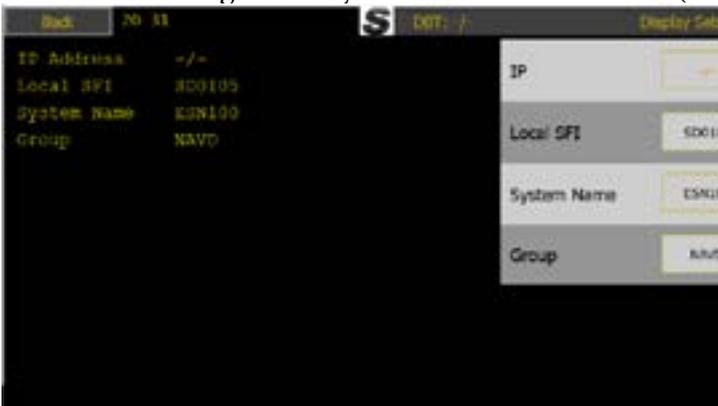
This standard requires a unique identifier for this equipment this is called the System Function Identifier (SFI). This is set by default to SD0105, but can and should be changed if more than one device on the network. The SFI is made up of 2 letters 'SD' as designated for an echosounder, and 4 digits from 0001 to 9999. This is used to allow the equipment to identify itself to other equipment, and to filter which messages are aimed for this device.
